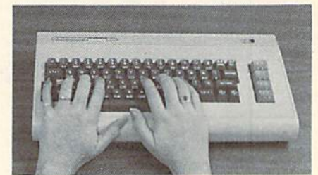
Pressing certain adjacent keys at the same time, such as Commodore-RUN/STOP, can erase all your text and restart the program.
